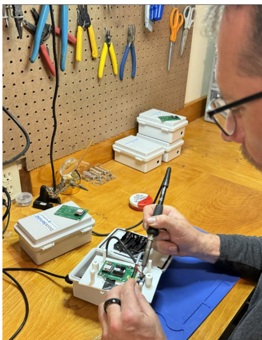
Noah Lottig assembling and soldering a DockSensIQ™ sensor at Trout Lake Station
