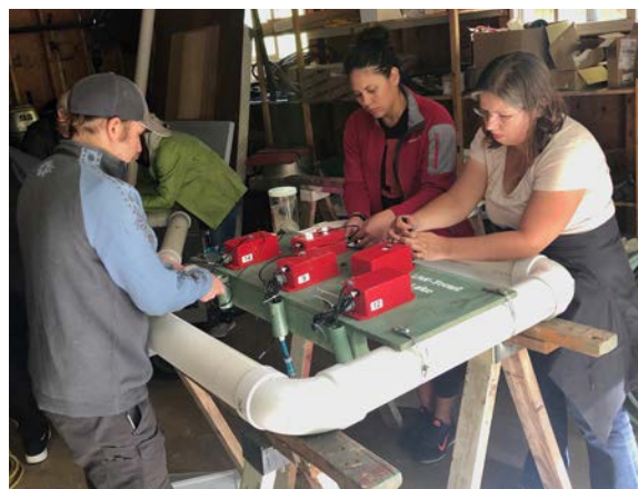
Attendees at a buoy building workshop at Trout Lake Station work attach sensors to an inexpensive buoy design. Photo: N. Lottig
